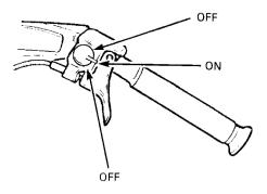
Turn ignition key clockwise until starter engages. Release key immediately engine has started. If engine does not start on first try, key must be turned fully back to OFF each time.
