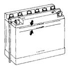
CAUTION: Do not allow cleaning solution to enter battery. It will destroy the chemical properties of the electrolyte.
