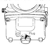
Re-install plug and connect fuel line. Check all fuel lines, replace if necessary.
