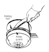
WARNING: When starting the vehicle in an emergency situation by the drive pulley, do not make a knot at the end of the emergency rope and do not reinstall the pulley guard.
