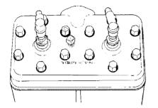
**IMPORTANT:** The engine head nut torque should be checked after the first 5 hours of operation.
