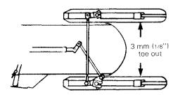
The handlebar should also be horizontal when the skis are pointed toward the front
