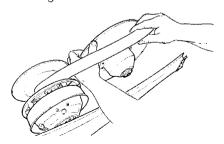
Slip the belt out from the drive pulley and remove completely from the vehicle. To install the drive belt, reverse the procedure.
