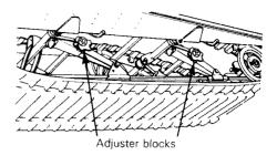
CAUTION: Always turn the left side adjuster blocks in a clockwise direction, the right side blocks in a counter-clockwise direction. Left and right adjuster blocks of each adjustment must always be set at the same elevation.
